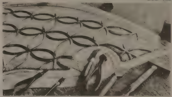
Figure 204: Construction of a stained-glass window. The craftsman has assembled a section of a large window on his glazing bench. Visible in the photograph are the design beneath the window and various tools for cutting glass and working the lead.
